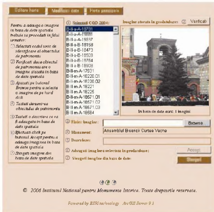
Figure 6. eGISpat Bucharest – the ability to add and delete image files to geodatabase
