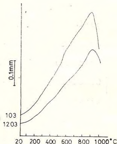
Fig. 12 — Dilatometric curves of limestones in Nucșoara Valley formation.
