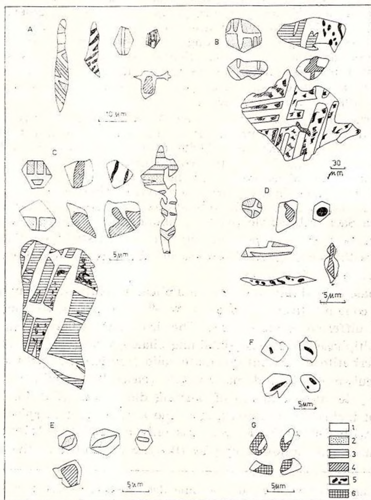
Fig. 3. — Types of inclusions in sphalerites: A-D, iron rich sph (10-15 wt.-% Fe); E, sph with 6 wt.-% Fe; F-G, iron poor sph (1.0-2.7 wt.-% Fe). The greater inclusions in B and C reflect the derivation of the coexisting minerals from the high T iss ; the po is grown in a phase resembling cp , not distinguishable from the cp of the laths (B); coexisting cb and mck developed on a sol-sol matrix with lanceolate cp laths suggesting a paramorphic transformation of a high T phase. The smaller inclusions contain only frozen assemblages, in which mck does not occur together with iss ( cpo ) as cb sometimes does (in B).
